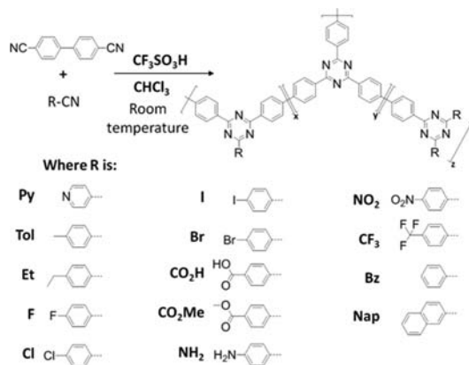
Figure 1. Synthesis of triazine-based MOP P1-R-X . 4,4'-Biphenyldicarbonitrile and a mononitrile aromatic functionality (R-groups) were trimerized to yield an insoluble polymer. Mononitrile functionalities were incorporated at 15% or 30% molar in the feed. The polymer may include three different repeat units: triazine rings with one adjacent R-group (x), triazine rings connected to three other triazines (y), or triazine rings connected to two R-groups (z).
